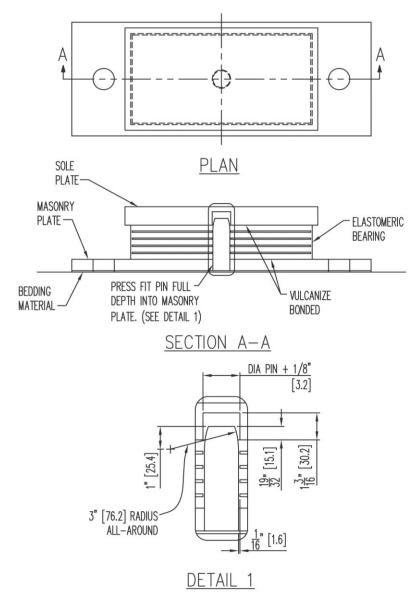
1. THE DIAMETER OF THE PIN SHALL BE CHECKED FOR SHEAR DUE TO HORIZONTAL LOADS. THE MINIMUM PIN DIAMETER SHALL BE 1.5" [38.1 mm].
