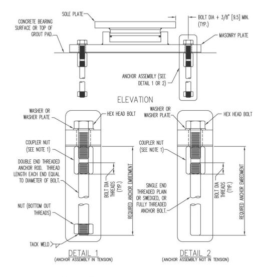
1. SPECIFY GRADE 'A' OR GRADE '2' COUPLER IF NO TENSILE FORCE ON ANCHOR BOLT. SPECIFY GRADE 'DH' OR '2H' COUPLER FOR TENSION ON THE ANCHOR ASSEMBLY.
